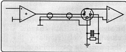
To connect an input to an unbalanced source, it is possible to connect pins 1 and 3 in the XLR plug at the amplifier end of the cable. However, a better method is to connect pin 3 to the shield at the source end of the cable, as this usually results in better hum and noise rejection. Balanced input connections are recommended whenever possible.
