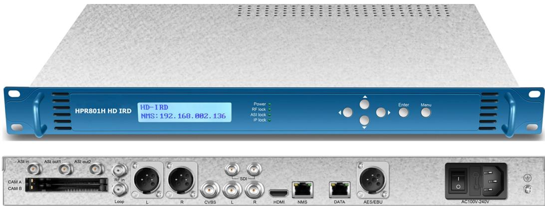
HPR801H HD IRD support AVS+/H.265/H.264/MPEG2 video decoding and DRA/AC3/EAC3/AAC/MPEG audio decoding. It support RF/ASI/IP input and 1080P/1080I/ 720P/576I/480I output resolution. The two CAMs/CIs accompanied and BISS modules can descramble the programs input from encrypted Tuner, ASI and IP.
