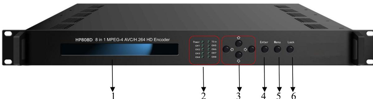
Indicate area: All indicators will light on when the device is on the current working state.
