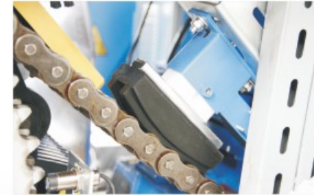
驱动链断裂保护 Driver protection strand breaks
