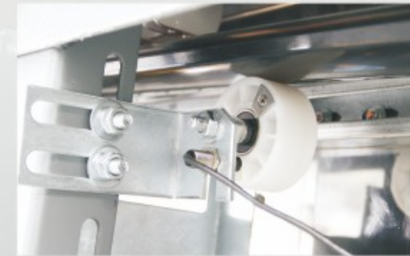
扶手带测速 Handrail speed
