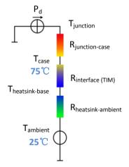
\*Thermal resistance is a heat property and a measurement of a temperature difference by which an object or material resists a heat flow.
