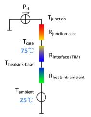
\*Thermal resistance is a heat property and a measurement of a temperature difference by which an object or material resists a heat flow. Geometric shapes are different, the thermal resistance is different.
