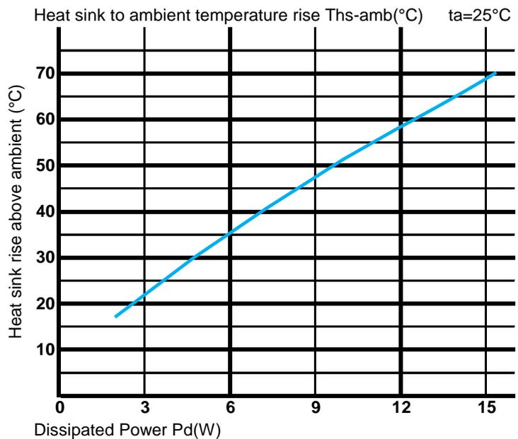
\*The aluminum substrate side of the package outer shell is thermally connected to the heat sink via TIM (Thermal interface material). MingFa recommends the use of a high thermal conductive interface between the LED module and the LED cooler. Either thermal grease, A thermal pad or a phase change thermal pad thickness 0.1-0.15mm is recommended.
