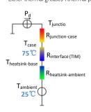
\*Thermal resistance is a heat property and a measurement of a temperature difference by which an object or material resists a heat flow. Geometric shapes are different, the thermal resistance is different. Formula:  $\theta = (Ths - Ta)/Pd$
