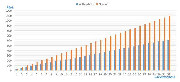
As demonstrated in the diagram above, the more channels are deployed, the more bandwidth saving is achieved. The bandwidth saving for 4 concurrent channels is 33.9% and for 32 channels is 43.8%. Please note that the test result shown is measured against a Single GoIP. This means that a GoIP-4 can only achieve a maximum bandwidth saving of 33.9% when all 4 channels are active.
