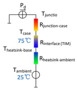
\*Thermal resistance is a heat property and a measurement of a temperature difference by which an object or material resists a heat flow.
