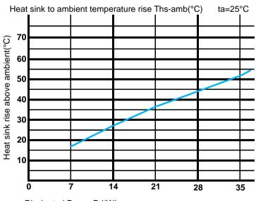
Dissipated Power Pd(W)
