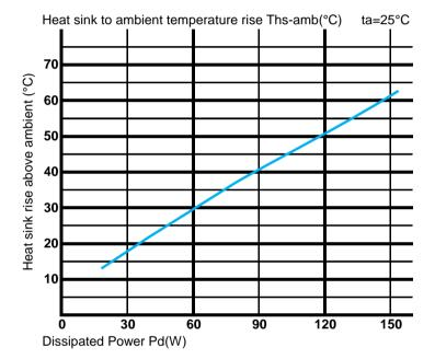
\*The aluminum substrate side of the package outer shell is thermally connected to the heat sink via TIM (Thermal interface MingFa recommends the use of a high thermal conductive interface between the LED module and the LED cooler. Either thermal grease, A thermal pad or a phase change thermal pad thickness 0.1-0.15mm is recommended.
