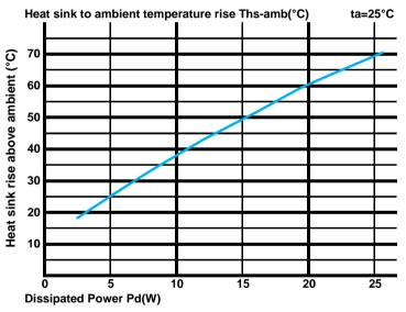
\*The aluminum substrate side of the package outer shell is thermally connected to the heat sink via TIM (Thermal interface material). MingFa recommends the use of a high thermal conductive interface between the LED module and the LED cooler. Either thermal grease, A thermal pad or a phase change thermal pad thickness 0.1-0.15mm is recommended.
