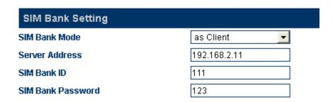
After the information of SIM Bank has been added on the server, the registration of server is completed only after the client-side mode has been enabled on the SIM Bank terminal and the card has been inserted.
