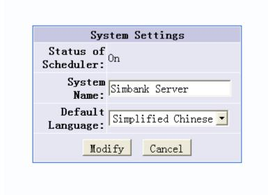
Status of Scheduler: Displays whether the background processes smb\_scheduler and xchanged run normally, and it is normal while "On" is shown.
